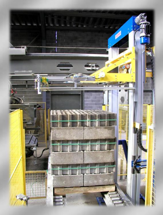
Fully-automatic strapping m chines for Brick & Concrete Pavers Industry
